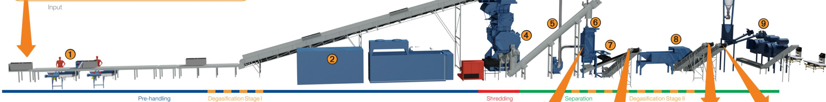
**1. Pre-handling.** The refrigerators are unloaded and pre-classified. The cords are cut off and the glass inserts are delivered to special containers. All CFC-gases, pentane gas and isobutan gas are extracted, and the compressors are dismantled.
